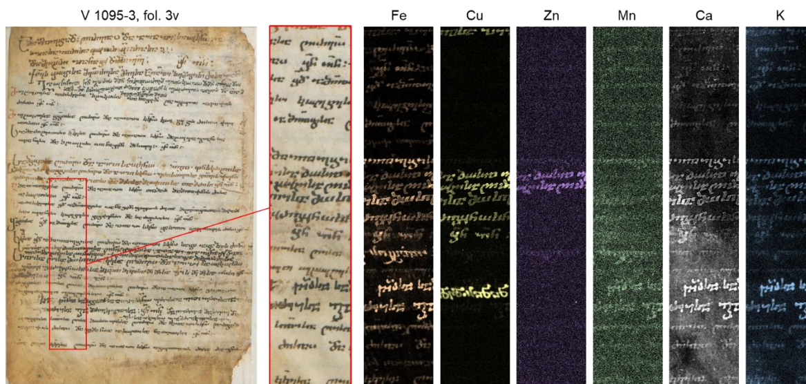
Fig. 9: XRF element maps of iron (Fe), copper (Zn), manganese (Mn), calcium (Ca), and potassium (K) for a scanned area on Leipzig, UL, V 1095-3, fol. 3v.
