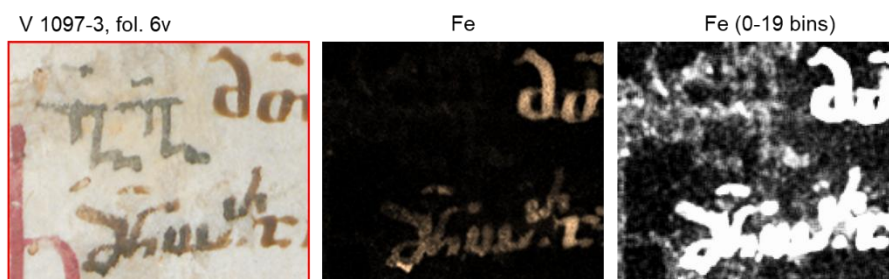
Fig. 11. XRF element map of iron (Fe) in standard visualisation (centre), and filtered by pixel averaging, black-and-white scale, and reduction to 20 bins (right) in order to highlight the weak iron signal of the red letter.
